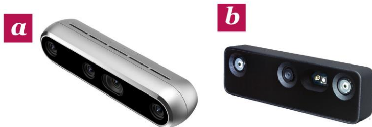
Figure 6 Stereo cameras and IMUs evaluated for the prototype: (a) Intel RealSense D455, (b) OAK-D Pro W, (c) Intel RealSense 435 and Intel RealSense T265 used as a pair.
