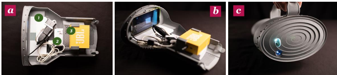
Figure 1 Detail views of the TRL4 prototype of the AR Magic Lantern: (a) top view, case open, (b) side view, case open, and (c) front view, case closed.
