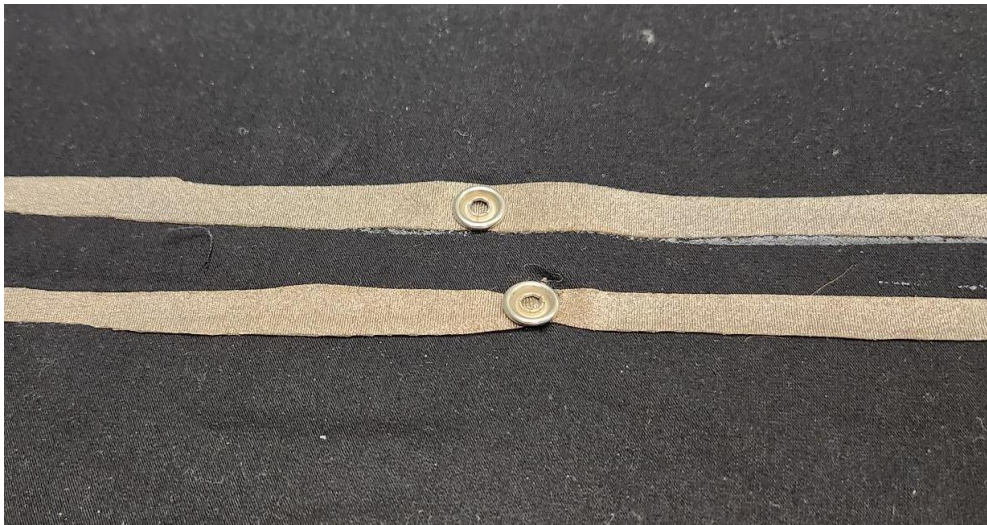
Figure 36 Conductive traces made of electrically conductive fabric strips
