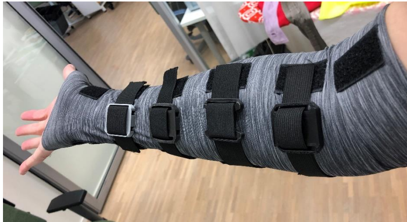
Figure 37 Thermo-haptic sleeve with attached Peltier elements and vibration motors that allows for the programming of thermal and haptic patterns such as a moving sensation by calling the actuators successively.
