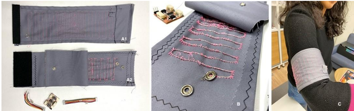
Figure 4 Prototype of wearable yarn-based heating pad for initial user testing. A1) Top of the heat pad. A2) Bottom of the heat pad with an additional fabric cover. B ) Metal snap buttons to connect the heating element to the control circuit. C) Prototype worn on the upper arm.
