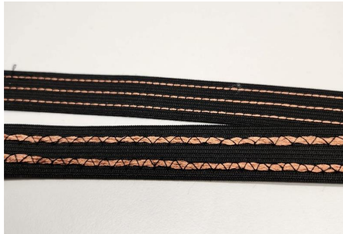
Figure 35 Conductive traces of various strengths made by sewing copper wires
